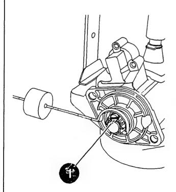
Checking clutch overrunning torque
